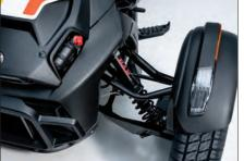
**FULL KYB HPG SHOCKS** Front and rear KYB HPG shocks with remote adjusters and 1 inch of extra suspension travel to optimize your ride
